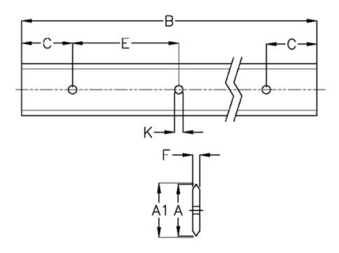
$\begin{array}{lll} A & = 76 \\ A1 & = 77.58 \\ B & = 2336 \\ C & = 43.0 \\ E & = 90 \\ F & = 9.43 \\ For bearing = J54 \end{array}$
